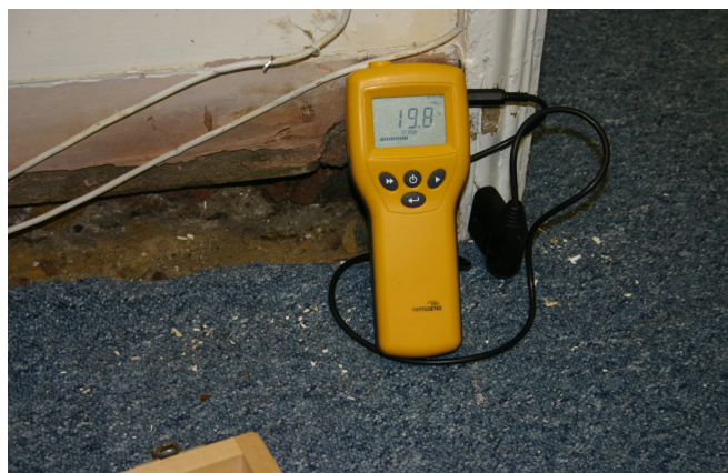
Figure 18: Electrical moisture meters have a role to play in diagnosing dampness problems when used in the correct hands. Photo: Douglas Kent
